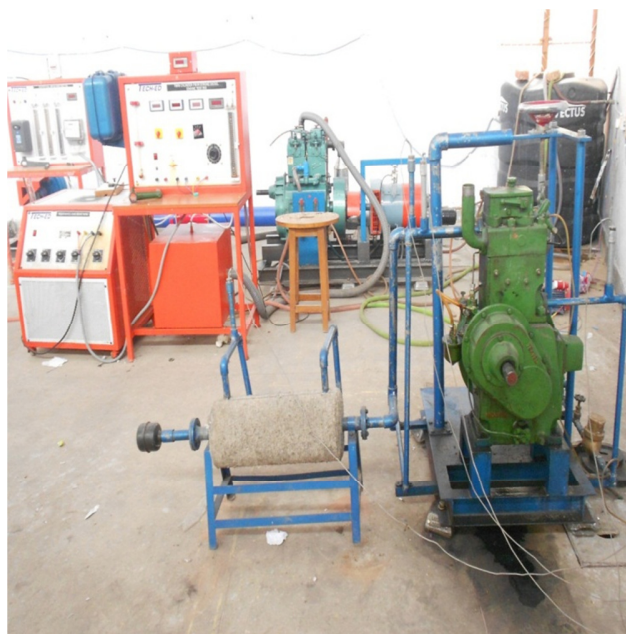
Fig.3.2 Engine set-up used for testing the fuel
